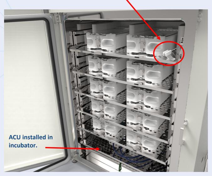
8. Attach magnet on glass door, aligned with shelf mounted sensor. Sensor will light red when properly aligned and powered.
