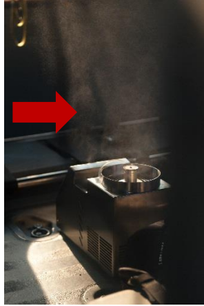
Phileas 20I actively decontaminating the cabin and cockpit area
