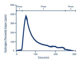
Phase 1 – Setup is user driven, whereby the user will need to enter the Service wrench icon on the Home screen, then the Decon program button, and follow all instructions on screen. This includes removing all cultures from the incubator, removing some water from the internal water reservoir with the provided removal syringe, adding 50%  $\rm H_2O_2$  to the internal water reservoir, mixing the solution with the removal syringe, and sealing the door with the Lock out tape warning label.
